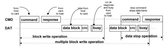
Figure 6.1.5: (Multiple) Block Write Operation
