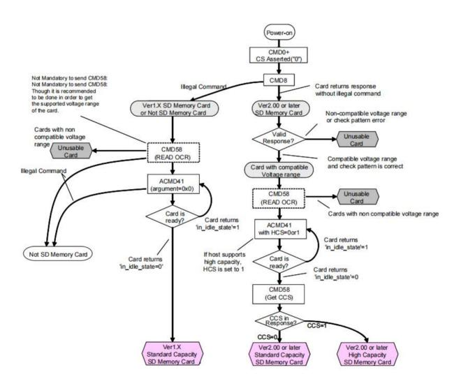
Figure 6.2.2: SPI Mode Initialization Flow
