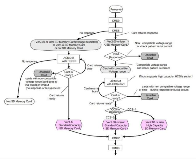
Figure 6.2.1: Card Initialization and Identification Flow (SD mode)
